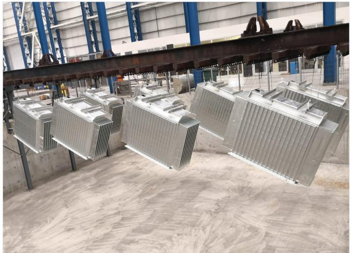
**ADS METAL A.Ş produces high quality HDG transformer tanks for long term corrosion protection needs for their customers according to ISO1461 Standards.**
