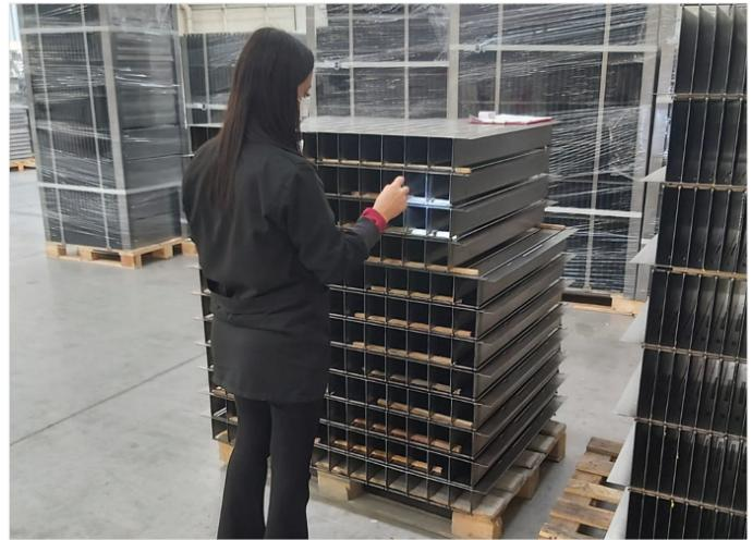
**Our quality team carefully checks each seams welding visually according to EN ISO 17637 standarts, dimention controls. In case of any defect found by our team is repaired sensitivly by Argon Welding technique. All reports are send to the costumer with the meterails.**
