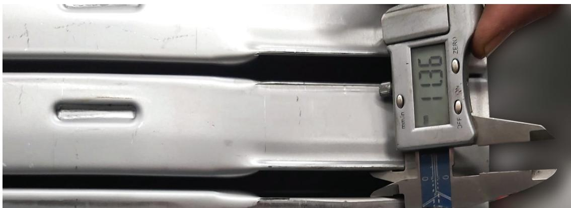
Super Onda Model corrugated walls gives for transformer designers more effective cooling chance by its revolutionary design. It provides an oil circulation inside the corrugated wall and increases the heat transfer rate.
